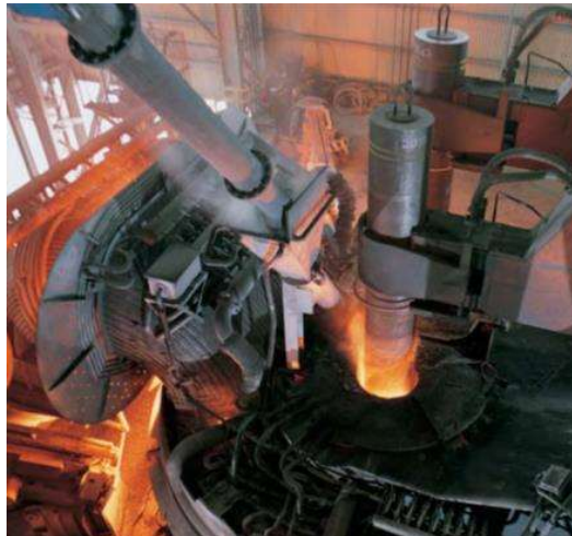
Figure 11. High-Carbon HDRI feeding the EAF at Ternium Monterrey
