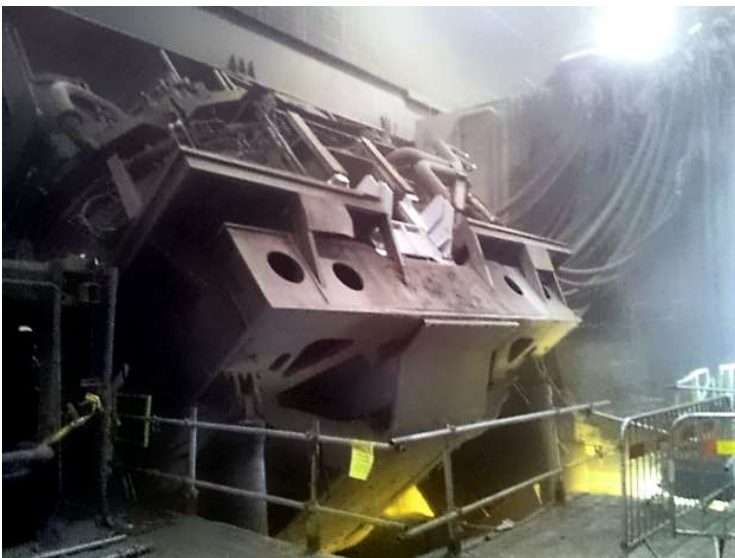
Fig. 2 – TENOVA EAF equipped with ABB ArcSave® @ Outokumpu Stainless AB, Avesta, Sweden.
