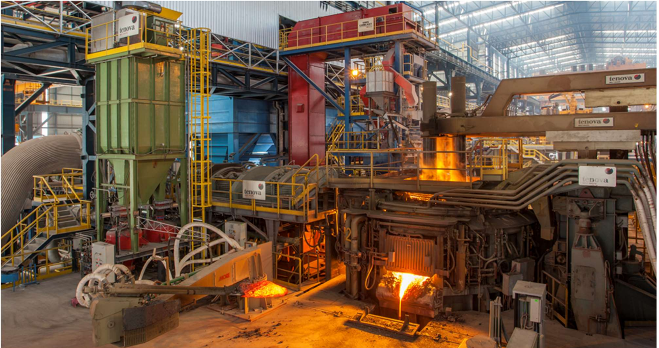
Fig. 1 – Flat bath operation of TENOVA Consteel® EAF @ Bangkok Iron and Steel Works, Bangkok, Thailand.
